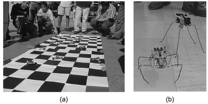
Fig. 1. Photos from the BEAM workshops. (a) Group of teachers test their fotopoppers in the January 2001 workshop. (b) Two *caminante* robots (a micro-core-based robot) are built by children in the January 2001 workshop.
